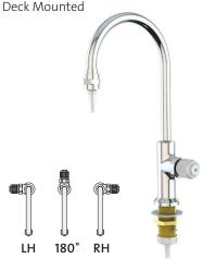
**Application:** Deck mounted faucet for distilled, deionized or reverse osmosis water. Faucet has exterior brass casing and interior lining of inert polypropylene. Pure water comes in contact only with inert plastic.
